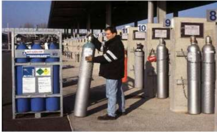
Air Liquide B50 200 bar 10 Nm 3 (= 0.9 kg H 2 )
